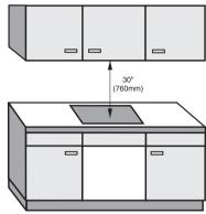
The minimum safety distance given by the hood manufacturer must be maintained between the cooktop and the hood above it. See the installation instructions of the hood for these safety measurements.
